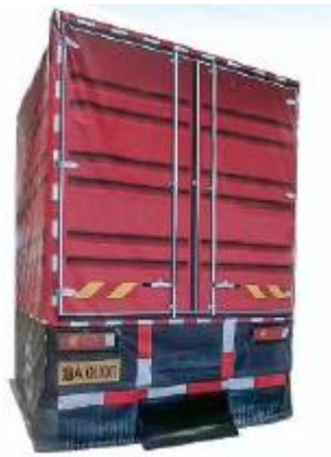
Fig. 5 Appearance of Flexible Truck Target
